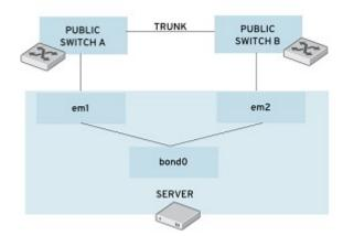
Figure 2.2.2: Ethernet Bonding
